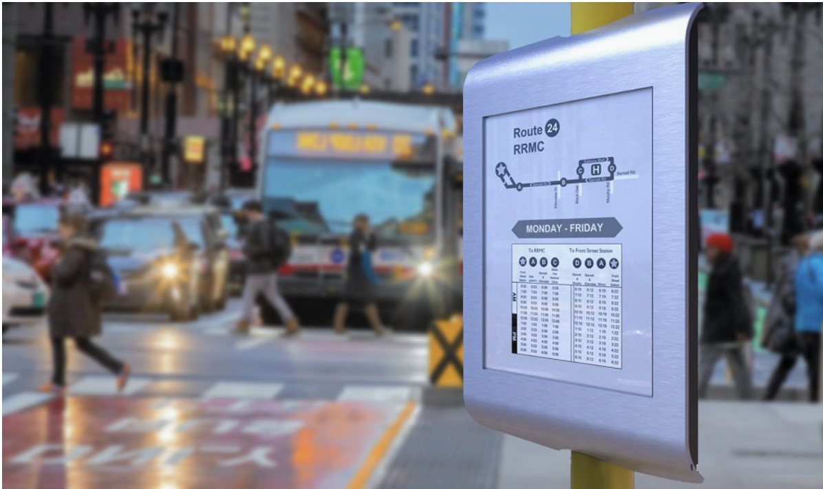
The GDS e-Tela solar-powered bus stop sign provides live updates on arrival times.
