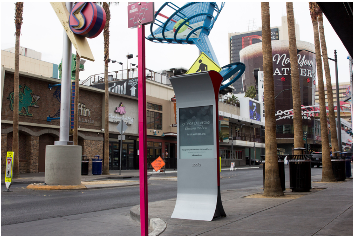
Soofa sign in downtown Las Vegas with 42" E Ink display Photo courtesy of Soofa
